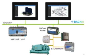
The use of touch-screen displays to manage entire floors and even small buildings is getting a common requirement in technical specifications. TAD panels perfectly fulfill these needs.
